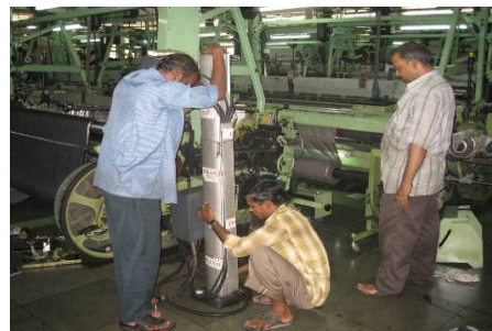
Loom parts being disassembled for diagnosis
