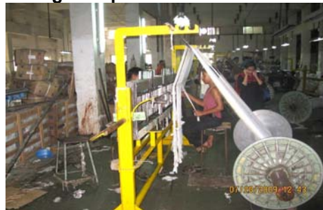
(2) Drawing the warp beam ready for weaving
