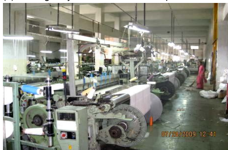
(3) Weaving the fabric on the weaving loom
