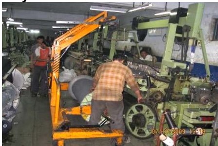
Warp beam being unloaded off a broken loom
