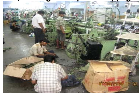
Parts being cleaned and replaced on jammed loom
