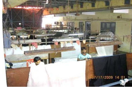
Workers spread cloth over lighted plates to spot defects
